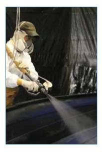
"With the quick-adjust on the cutter head, instead of stopping and taking the cover off, you simply adjust the level on the cutter head to reduce long hairs of fiberglass. This saves time and money on parts. I really love that feature."
