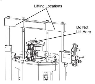
Fig. 2: Lifting the Machine
