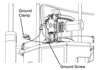
Fig. 3: Grounding Connection
