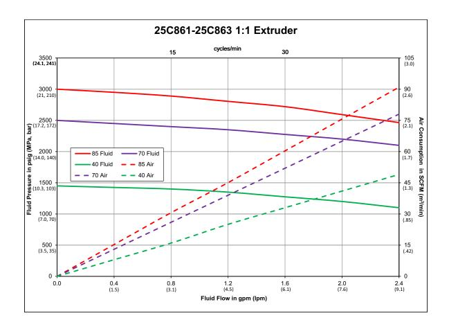
**NOTE:** Performance is measured using 10 weight oil.
