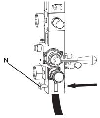
Fig. 4: Open Main Air Slider Valve
