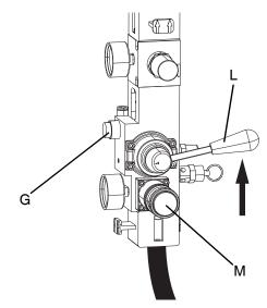
Fig. 9: Air Controls for Changing Pails
