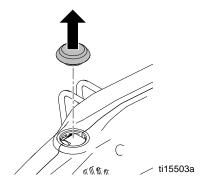
4. Use tool (supplied) to loosen and remove outlet valve fitting. Make sure old o-ring, seat, outlet valve, and spring are out of pump outlet cavity.
