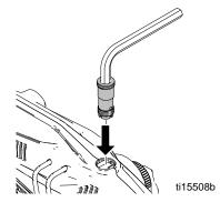
2. Press outlet valve fitting access plug.
