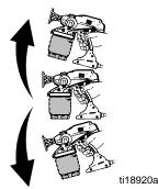
8. Disconnect trigger lock and trigger sprayer for approxi mately 15 seconds. Engage trigger lock.
