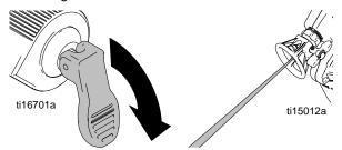
**IMPORTANT!** For best results, do not spray more than one cup of water through the tip while cleaning. If more flushing is needed, remove the tip from the sprayer.
