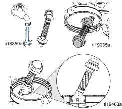
6. Clean material cup if not using a liner, and fill with water or appropriate flushing fluid.
