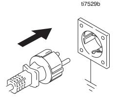
2. Do not use sprayer if electrical cord has damaged ground prong.
