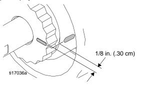
4. Position pressure control knob in fully clockwise position and press firmly onto retainer.
