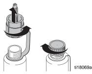
6. Attach flexible suction tube and material cup. Push valve DOWN to spray position.
