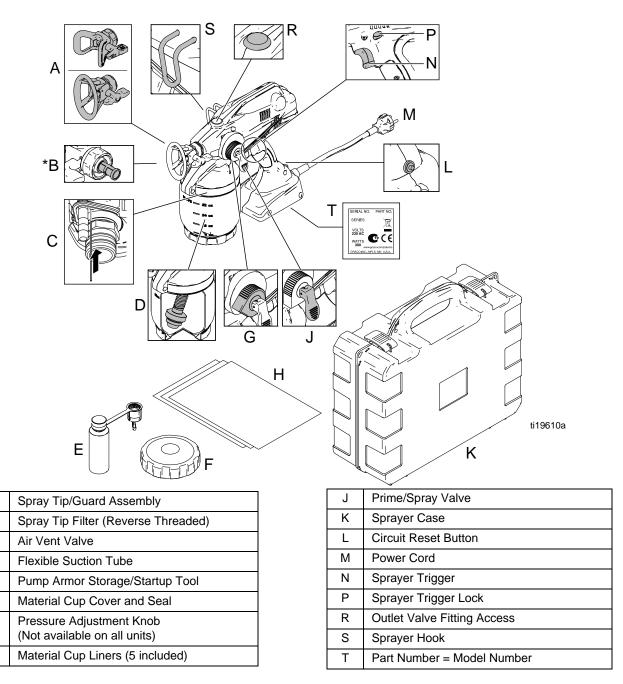
**\*NOTE:** Spray tip filter is reverse-threaded. Turn left (or counter-clockwise) to tighten, turn right (or clockwise) to loosen.
