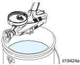
4. Insert Pump Armor nozzle over material inlet and push firmly until it stops. Squeeze cleaning bottle until Pump Armor flows out drain tube.
