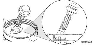
**NOTE:** If the sprayer is angled or tilted too far, the flexible suction tube will lose contact with the material and the sprayer will stop spraying.
