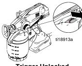
Trigger Unlocked (red ring is visible)
