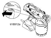
6. Put prime/spray valve UP to release pressure.
