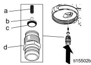
Hold inlet in place and turn sprayer upside-down. Remove inlet valve fitting and visually check to see that inlet valve has seated correctly.
