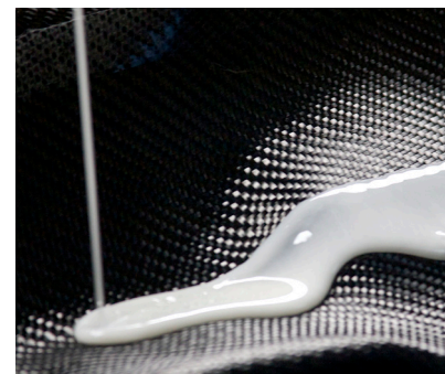
Spraying resin premix to a carbon fiber preform
