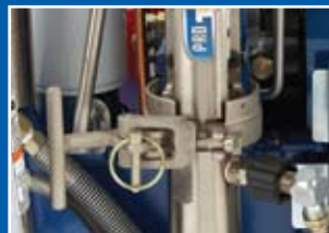
Exclusive ProConnect System, no-tools pump removal and installation.
