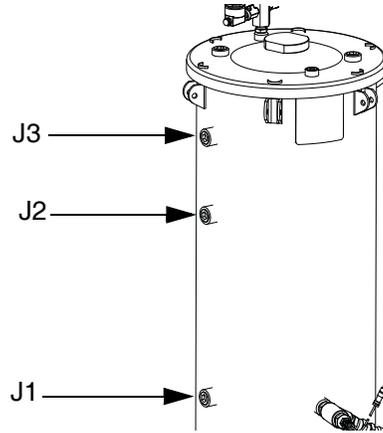
**FIG. 8: Tank Ports**
