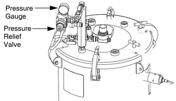
**FIG. 13: Tank Pressure Relief**
