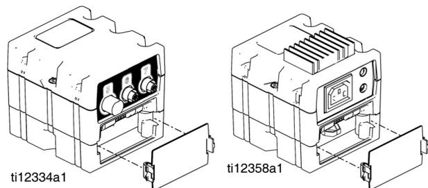
**FIG. 14: Remove Access Cover**
