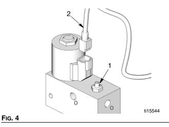
**NOTE:** If using one of the BSPP Vent Valve Kits, install adapter (7) into pump element prior to installing pump element fitting (c) then continue installation, Step 6.
