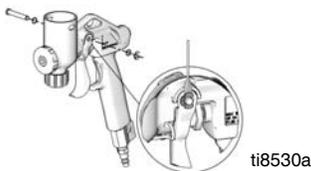
9. Pull trigger and replace nozzle.
