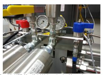
Fig. 27: HFR Manifold Valves in the Manual Circulation Positions
