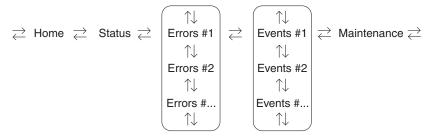
Fig. 25: Run Screens Navigation Diagram
