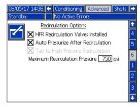
Fig. 28: HFR Setup Advanced #6 Screen - Circulation Options
