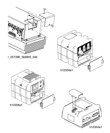
Fig. 17: Remove Access Cover
