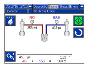
Fig. 31: Main Operator Mode Run Screen, with Circulation Option.
