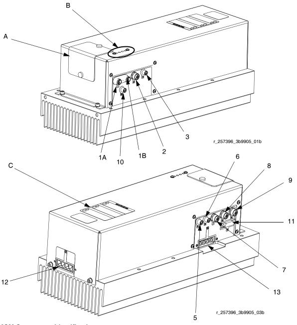
Fig. 4: MCM Component Identification
