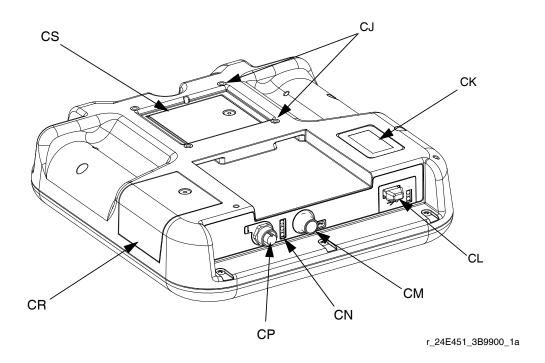
Fig. 20: ADM Component Identification - Rear
