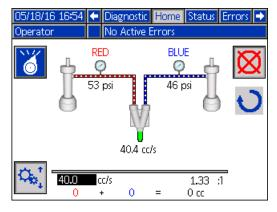
Fig. 35: Changing Flow Rate for a Manual Circulation Dispense
