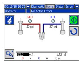
FIG. 33: Main Operator Mode Run Screen, with Circulation Option Selected.
