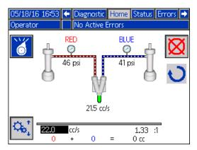
Fig. 34: Operator Mode Run Screen while Manually Circulating Material.
