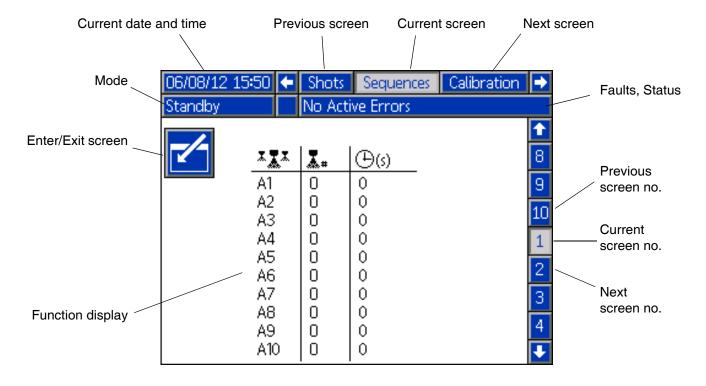
Fig. 7: Main Display Components
