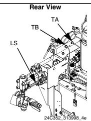
Fig. 2: Component Identification, Heated Model shown with shrouds removed
