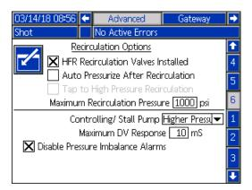
HFR Circulation Valves Installed - Activate this feature if the Semi-Automatic Circulation Kits are installed. If checked, the hydraulic level sensor option provided on Setup System Screen #2 will not be available. Do NOT check this box if air driven circulation valves are not installed (default).
