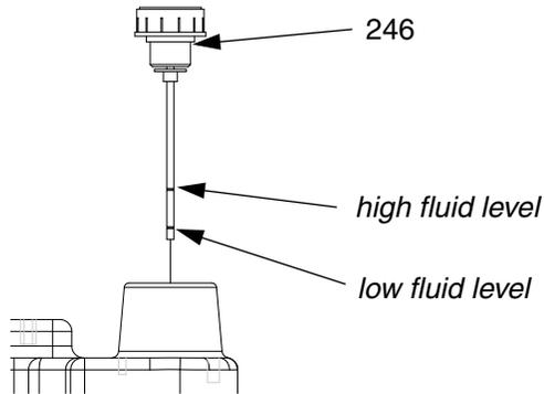
**FIG. 23: High and Low Fluid Level Marks**
