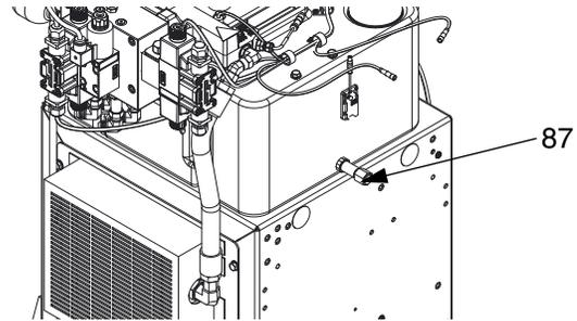
**FIG. 24: Drain Cap**
