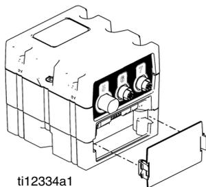
**FIG. 36: Remove Access Cover**
