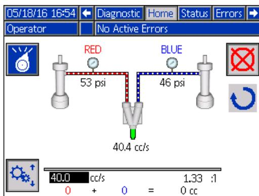
**FIG. 35: Changing Flow Rate for a Manual Circulation Dispense**
