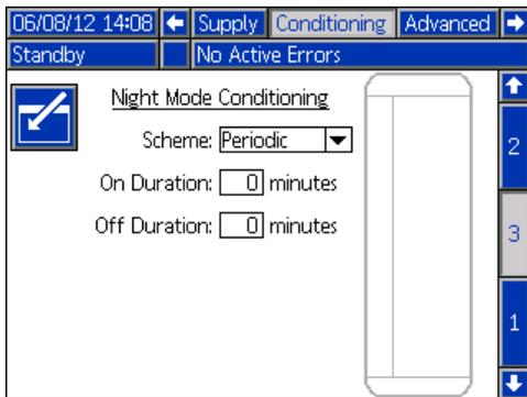
Night Mode is available for full recirculating systems (L-Head, S-Head, and S-Head w/ Prox valve options), and systems with semi-automatic recirculating kits installed (refer to **Appendix H- Circulation** on page 111 for recirculating kit details).
