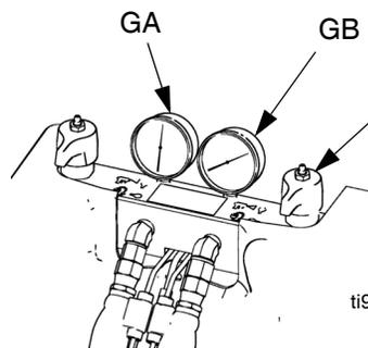
In this example, B (Blue) side pressure is higher, so use the B (Blue) side valve to balance pressures.
