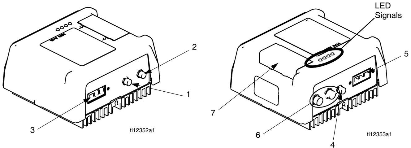
**FIG. 9: High Power Temperature Control Module Sensor Connections**
