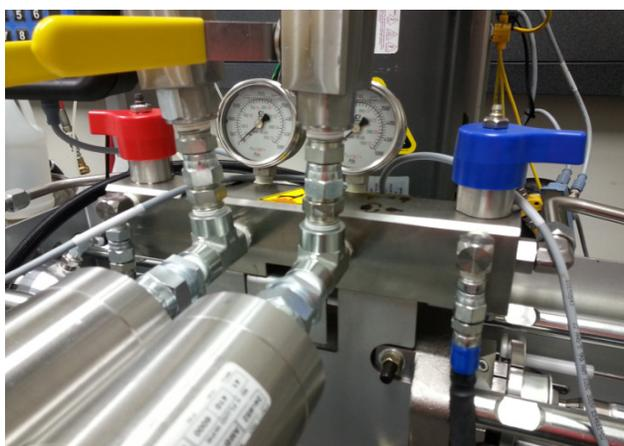
**FIG. 27: HFR Manifold Valves in the Manual Circulation Positions**
