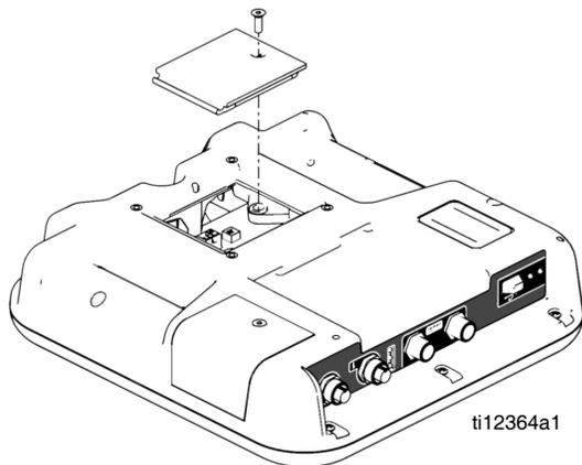
3. Remove the old battery and replace with a new CR2032 battery.
