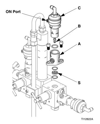
Fig. 4. Valve Adapter and Seat
