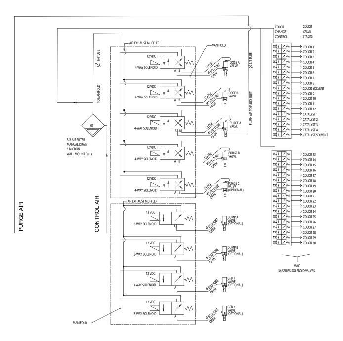
Fig. 3. System Pneumatic Schematic
