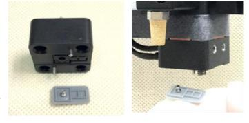
4. After the diaphragm is inserted, the nozzle plate can be attached to the heater
