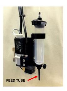
3. Slip the feed tube onto the barb end of 4. Install the receiver head. the nozzle plate.
