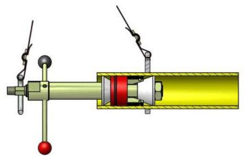
2. Once the plug cannot be moved within the pipe, rotate the handles the number of turns specified in **TABLE 2**, for the pipe size being tested.
