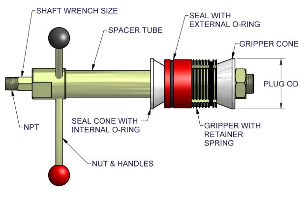
Figure 1: GripTight PE Test Plug
