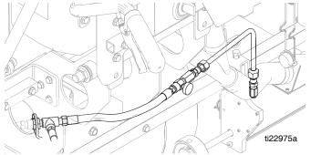
5. Attach hose tee to fitting (21mm).
