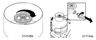
2. Remove plug and copper gasket (ferrule) from fitting.
