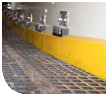
PU sideliners with chamfer top for Metso MF, mining screens
