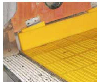
PU sideliners for flat top for CVB or TS screens
