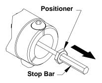
Fig. 21: Valving Rod Removal
