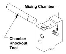
Fig. 22: Mixing Chamber Removal
