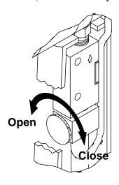
Fig. 7: Air Valve Adjustment
