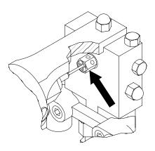
Fig. 8: Felt Wiper
