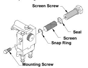
Fig. 17: Filter Screen Assembly
