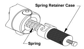
Fig. 20: Retainer Case Removal
