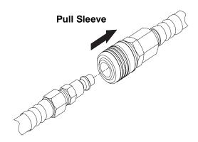
Fig. 5: Air Hose Connection
