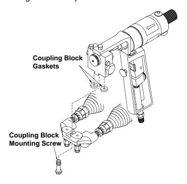
Fig. 3: Coupling Block
