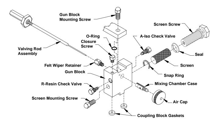
Fig. 2: Centerline Components
