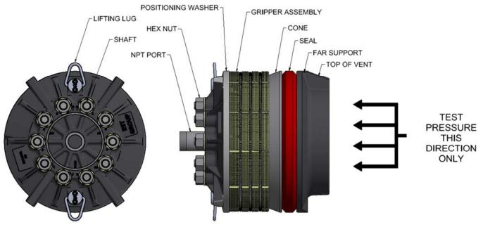
**GripTight MAX High Pressure Test Plug**
