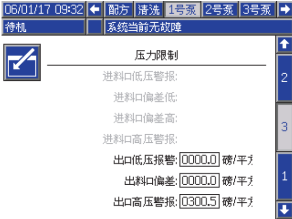
Figure 51 泵屏幕 3，已禁用压力监控
