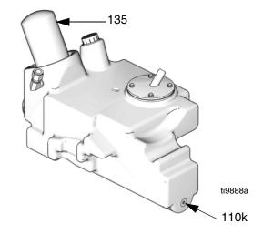
FIG. 16: Change Hydraulic Fluid and Filter
