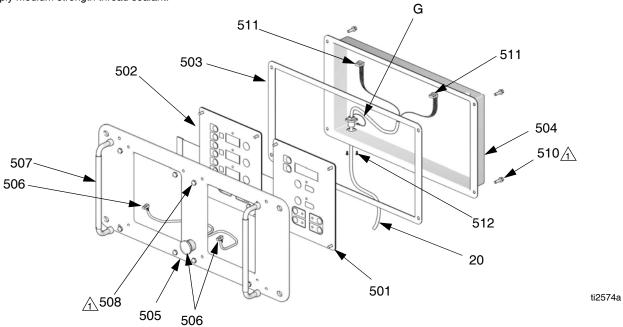
Detail of Membrane Switches and Display Boards
