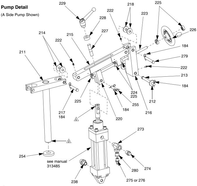
$\Lambda$  Apply blue Loctite and torque to 250 ft-lbs (337.5 N•m).
