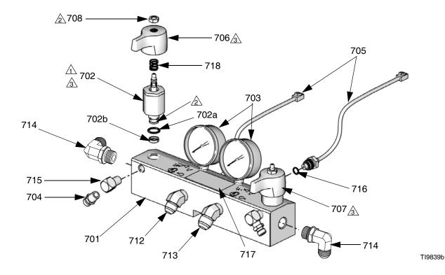
Qty Description Ref. Part 1 701 247837 MANIFOLD, fluid 2 702† 247824 VALVE, drain cartridge 1 702a† 158674 . O-RING 1 702b† 247779 . SEAL, seat, valve 2 703 102814 GAUGE, pressure, fluid 2 704 162453 FITTING, 1/4 npsm x 1/4 npt 2 705 24K999 TRANSDUCER, pressure, control 1 706 247788 HANDLE, red 1 247789 HANDLE, blue 707 2 708† 112309 NUT, hex, jam 1 712 117556 NIPPLE, #8 JIC x 1/2 npt 1 713 117557 NIPPLE, #10 JIC x 1/2 npt
