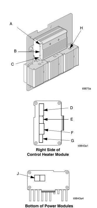
FIG. 9: Temperature Control Module Connections
