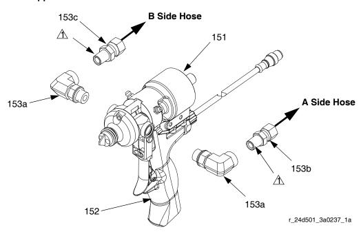
Apply anaerobic pipe sealant.
