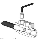
Fig. 9: Insert Wire and Setscrew
