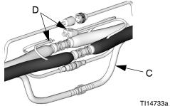
**Dual Heat Zone with A and B Heated Hose**
