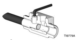
Fig. 10: Torque Setscrew
