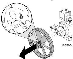
**NOTE:** Make sure key is in place before installing new pulley.
