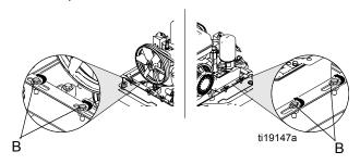
5. Loosen two belt tensioning bolts (C) to take tension off of belt. Loosen only until belt can be removed.
