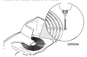
3. Once ridge has been drilled away on rivet, the remaining portion can be pushed through hole.
