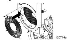
Close belt shroud with new fan grill onto unit.
