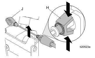
3. Replace original gun arm assembly with new gun arm assembly.
