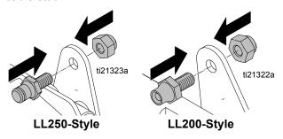
6. Replace old gun bracket with new bracket assembly (T).
