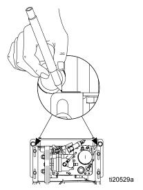
4. Use 9/16 in. wrench to loosen (but do not remove) four bolts (B) that secure hydraulic reservoir system to base plate.
