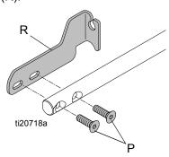
4. Replace with LL200 bracket (S). Push all the way forward in slots and tighten Allen heads (P).
