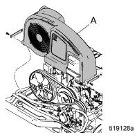
3. Before loosening belt assembly, mark location of hydraulic reservoir against stationary base.
