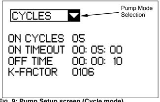
FIG. 9: Pump Setup screen (Cycle mode)
