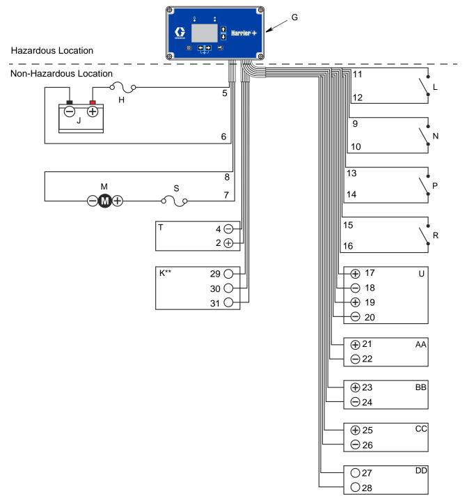
FIG. 2: Typical 12 or 24 VDC Installation
