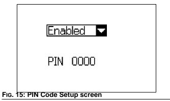
The PIN Code Setup screen allows you to enable a PIN Code Entry screen (see FIG. 16) that prevents access to the Configuration screen (see FIG. 6) without the correct PIN Code.
