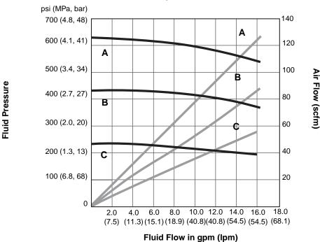
Stainless Steel 1000cc Pump with NXT Model 3400 Air Motor
