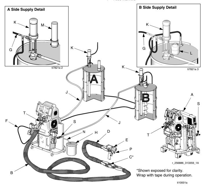
Fig. 2: Typical Installation, without circulation
