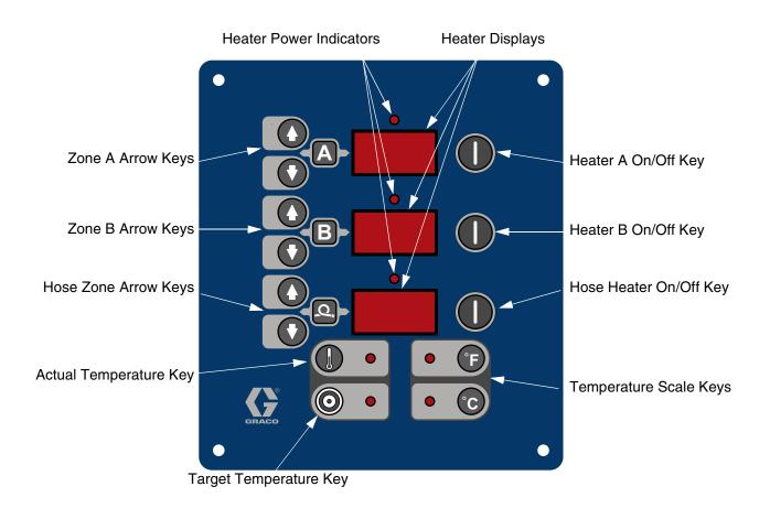
Fig. 5. Temperature Controls and Indicators
