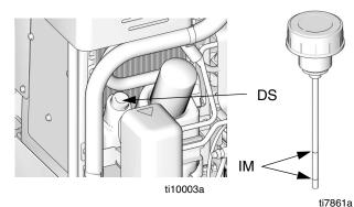
Change break-in oil in a new unit after first 250 hours of operation or within 3 months, whichever comes first. See Table 4 for recommended frequency of oil changes
