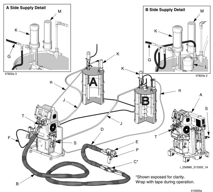
Fig. 1: Typical Installation, with circulation
