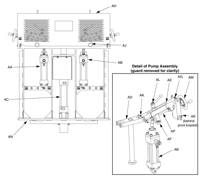
Fig. 4: Front View of Pump Assembly
