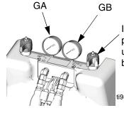
In this example, B side pressure is higher, so use the B side valve to balance pressures.
