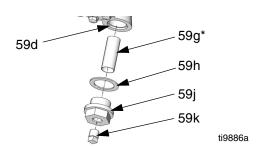
Fig. 11: Fluid Inlet Strainer
