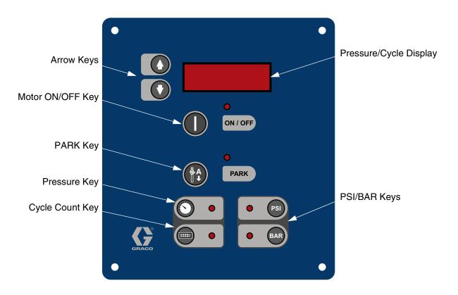
Fig. 6. Motor Controls and Indicators
