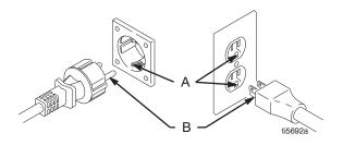
Do not use sprayer if electric cord has a damaged ground prong (B). Only use an extension cord with an undamaged 3-prong plug.
