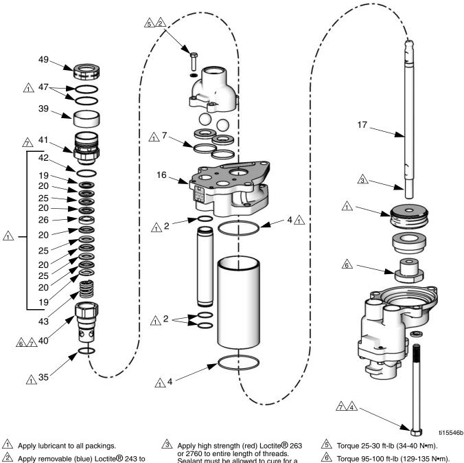
Apply removable (blue) Loctite® 243 to entire length of threads. Sealant must be allowed to cure for a minimum of 12 hours before use.
