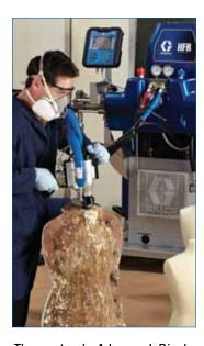
The system's Advanced Display Module (ADM) allowed Ronis to program multiple pour shots for multiple size molds. This eliminated downtime between line changeovers, increasing overall productivity and uptime. Having the ADM available in Spanish was a substantial added benefit for this facility.
