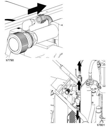
5. Remove four belt cover screws (79), washers (78) and grommets (80) (2 each side).
