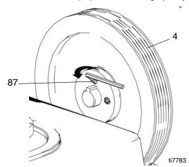
9. Remove pulley (4) from hydraulic pump shaft.
