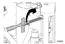
3. Attach hoses (100, 101) to head (75). Torque to 450 ± 10 in-lb (50.84 N•m).
