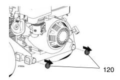
4. Insert plugs (120) in upper frame handle tubes (a).
