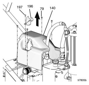
3. Remove compensator screws and separate compensator and adapter block.
