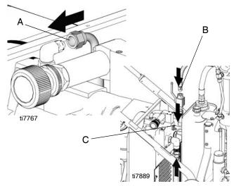
10. Install cover (140) and with four screws (79). Torque to 25-30 in-lb (2.8 - 3.4 N•m). Install pump handle cover (196) with screw (197).
