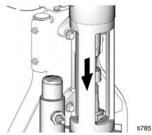
2. Tighten power head bolts (7). Torque bolts to  $400 \pm 10$  in-lb ( $45 \pm 1$  N•m).
