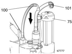
4. To purge air from hydraulic lines, increase pressure enough to start hydraulic motor stroking and allow fluid to circulate for 15 seconds. Turn pressure down. Turn prime valve horizontal (closed).
