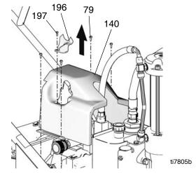
Unscrew suction line connections to hydraulic pump. Place a container under hoses to catch any dripping oil.
