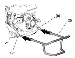
6. Install sleeve screws (143) in lower frame tubes.
