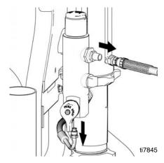
3. Loosen filter housing fitting (110) until housing and remove housing from pump.
