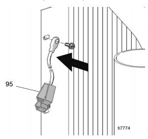
4. Replace bar and screws. Torque to 25-30 in-lb (2.8-3.4 N•m).
