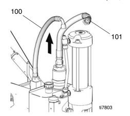
7. Remove cooler line from reservoir (64).
