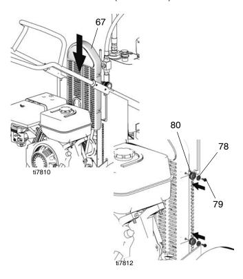
9. Install suction lines. Tighten fittings. Torque fitting A to  $225 \pm 10$  in-lb ( $25.4 \pm 1.1$  N•m). Fitting B to  $450 \pm 10$  in-lb ( $50.1 \pm 1.1$ . N•m). Fitting C to 225 in-lb (25.4 N•m).
