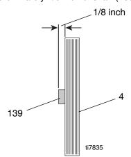
6. Replace set-screws (87). Tighten and torque to  $60 \pm 2$  in-lb ( $6.8 \pm 0.2$  N•m).
