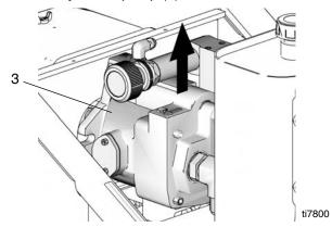
12. Remove fittings (30, 34, 35) from pump (3) and set aside to use on the new pump.
