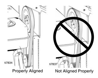
**NOTE:** If belt is not aligned properly, to adjust belt, slowly pull engine recoil while at the same time pushing or pull ing belt to reposition over pulley.
