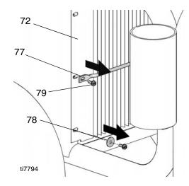
5. Remove coil (72) from sprayer frame.
