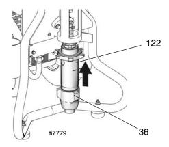
3. Hand tighten jam nut (122). Then tighten securely 1/8 to 1/4 turn with hammer or torque to 330 ft-lb (447.4 N•m).
