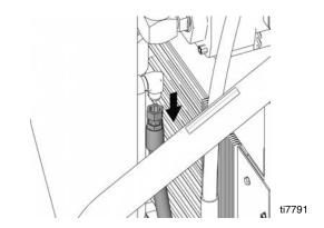
8. Remove two top bolts (86) and two bottom nuts (84) securing reservoir (64) to frame.
