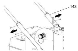
2. Pull handle assembly (25) out of upper frame tubes (1).
