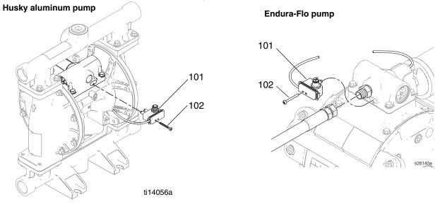
3. Connect the DataTrak cable to the 5-pin connector on the reed switch. Reconnect the air line to the motor.
