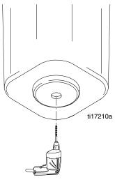
2. Assemble gasket (4) to fitting (5) and insert through 3 in. hole as shown below.
