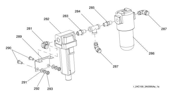
$\triangle$  Apply thread sealant and PTFE thread tape to all male npt threads as needed.
