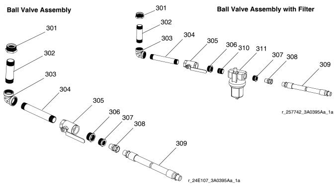
$\triangle$  Apply thread sealant and PTFE thread tape to all male npt threads as needed.
