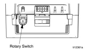
Fig. 6: Adjust Rotary Switch
