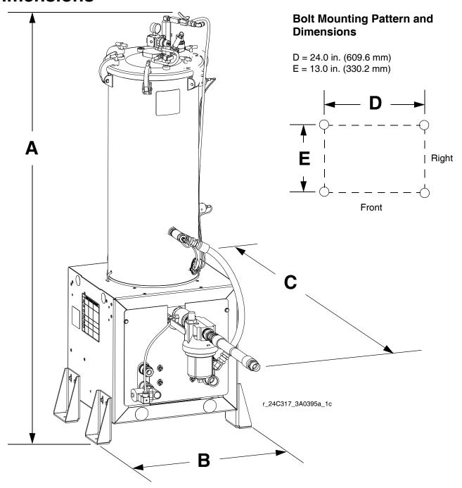
A = 83.0 in. (2108 mm); 38L/75L tanks with agitation
