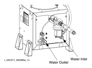
Fig. 10: Level Sensor Assembly
