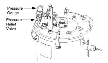
Fig. 13: Tank Pressure Relief
