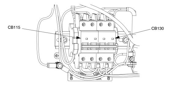
Fig. 2: Component Identification - Circuit Breakers
