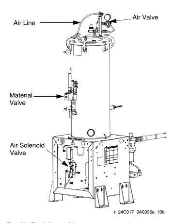
Fig. 11: Tank Assembly
