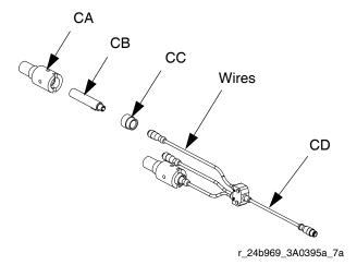
Fig. 7: Level Sensor Assembly
