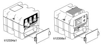
Fig. 14: Remove Access Cover
