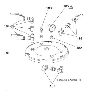
Apply thread sealant and PTFE thread tape.
