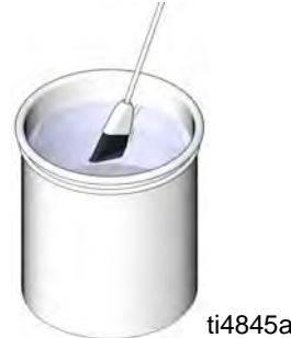
Fig. 14: Use solvent-dipped soft-bristle brush
