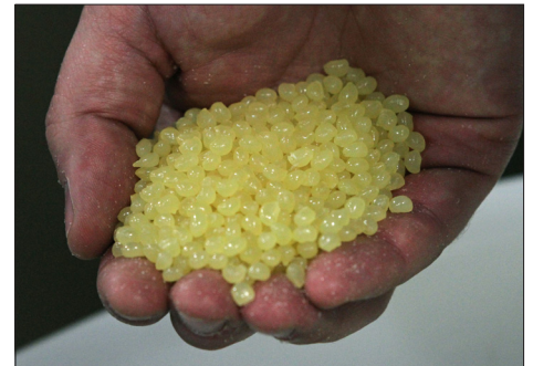
This pelletized adhesive is used in a new hot-glue process being used at Summit Brewing to seal boxes.
