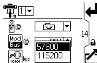
Figure 48 Set Baud Rate (Bits Per Second)
