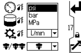
Figure 57 Select Desired Pressure Units
