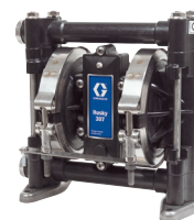
Husky 307 3/8 in (9.4 mm) connection Max flow: 7 gpm (26 lpm) Polypropylene, acetal
