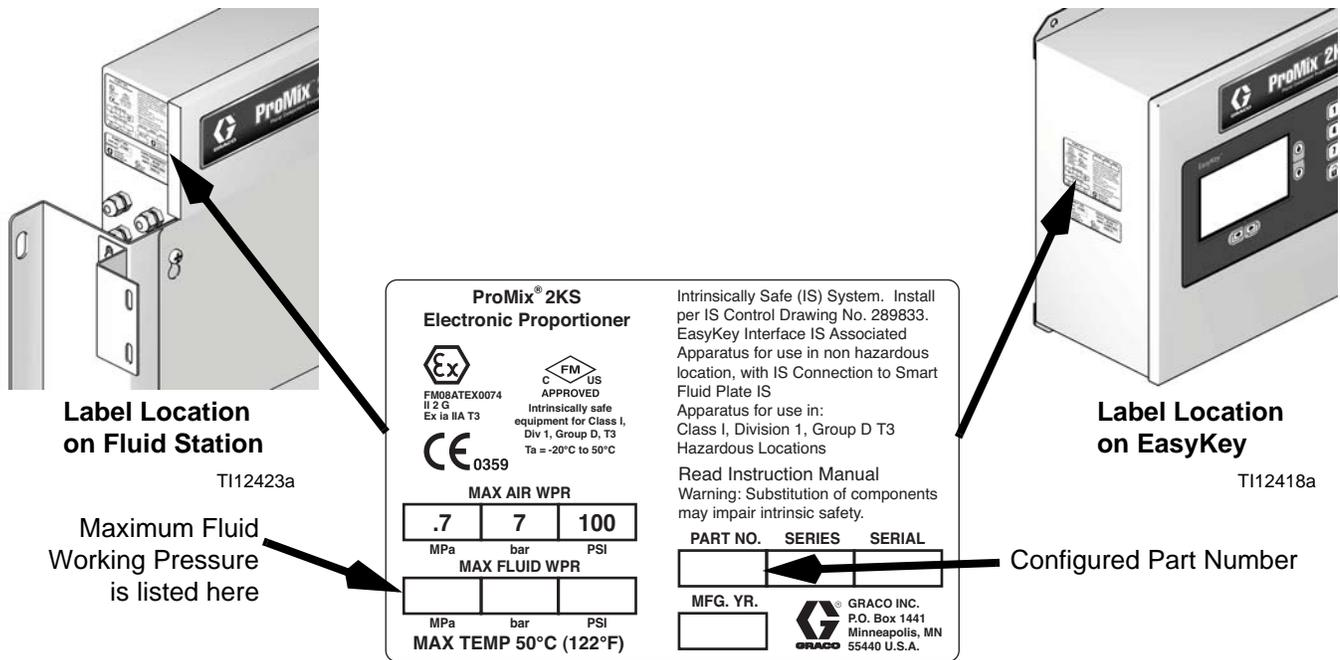
FIG. 1: Identification Label, Automatic Wall Fluid Station Systems
