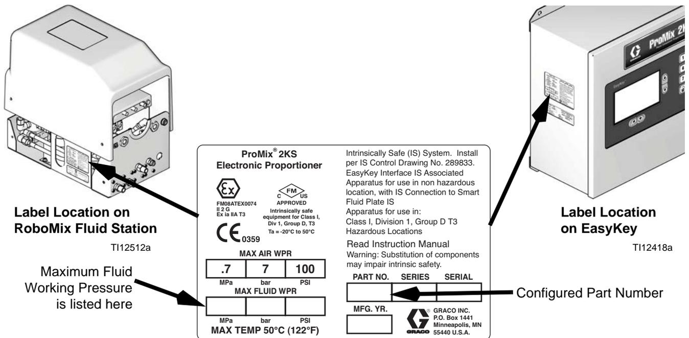
FIG. 2: Identification Label, Automatic RoboMix Fluid Station Systems
