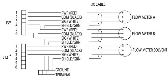
\*Connectors on Fluid Station Control Board
