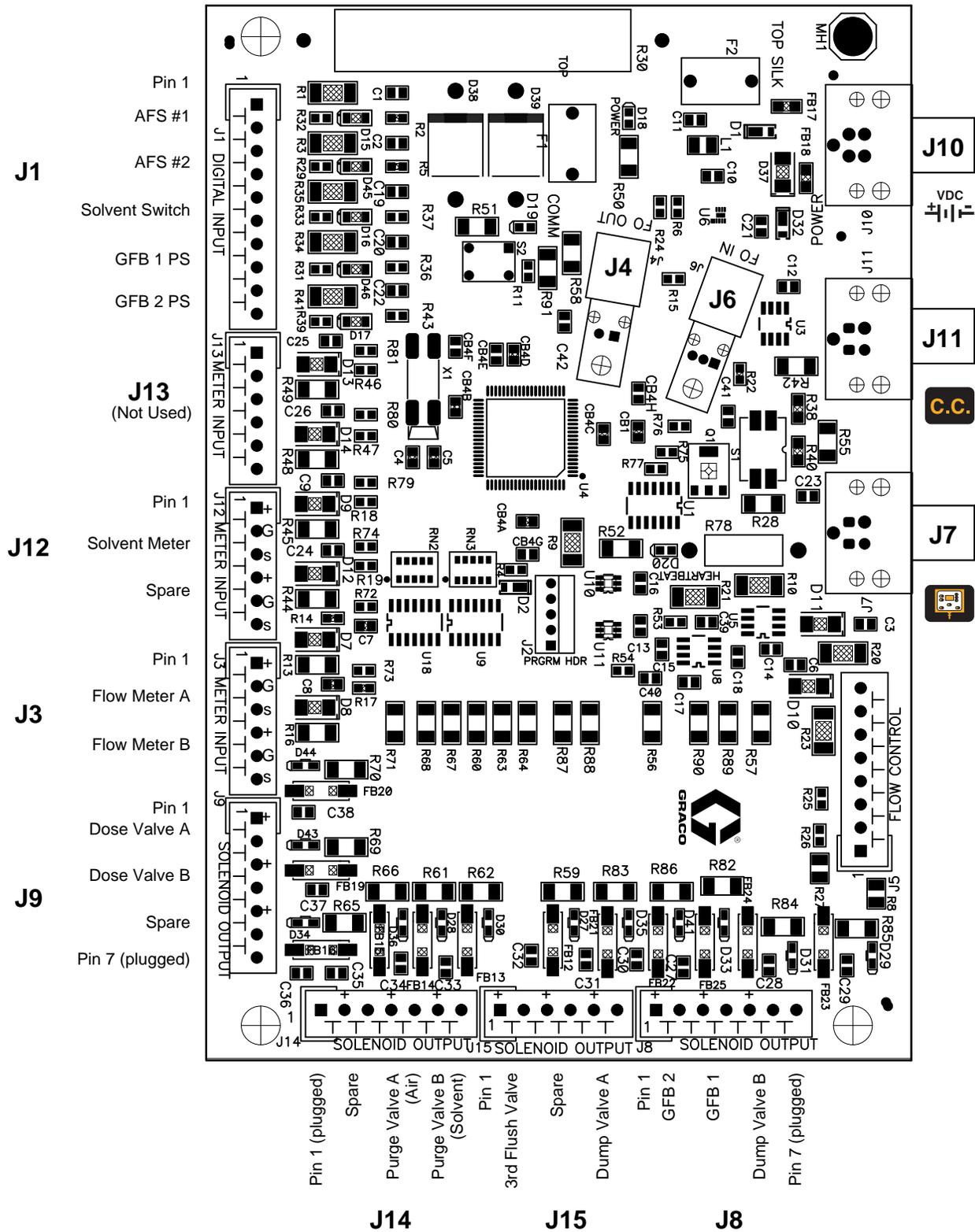
Fig. 12: 255765 Fluid Station Control Board Input/Output Connections
