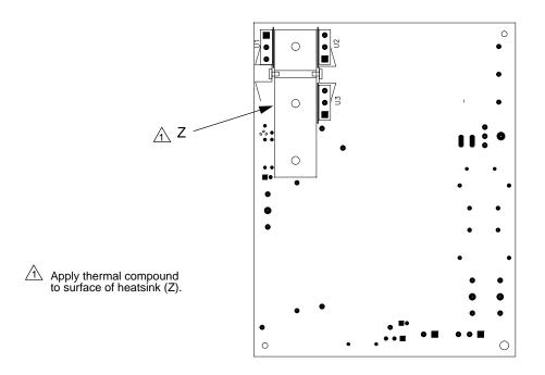
Back of Barrier Board, showing Heatsink (Z)
