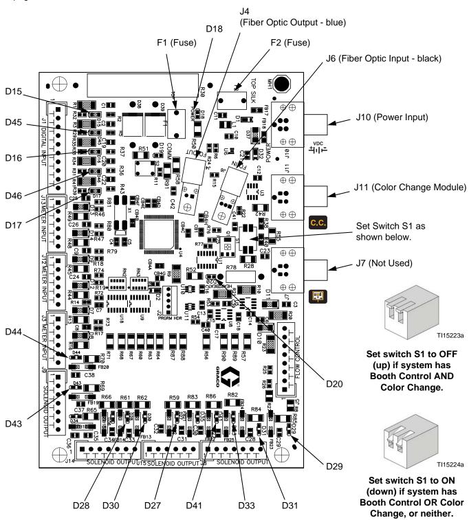
Fig. 11: 255765 Fluid Station Control Board Indicators
