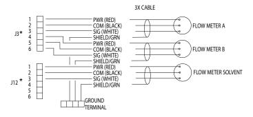
\*Connectors on Fluid Station Control Board
