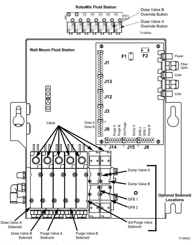
Fig. 5: Fluid Station Board and Solenoids
