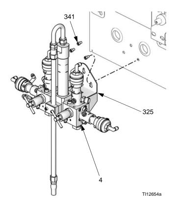
Fig. 25: Fluid Manifold
