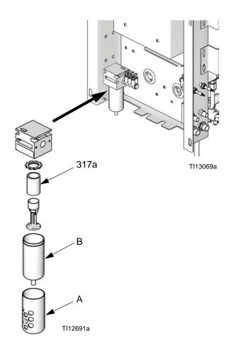
Fig. 19: Replacing Air Filter Element
