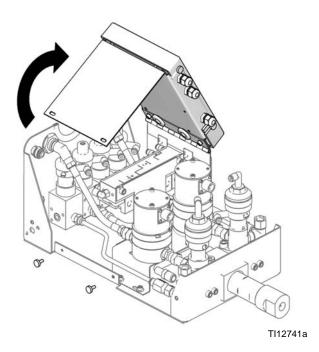
Fig. 30: Accessing Solenoids and Meters
