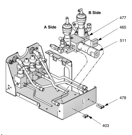
Fig. 34: RoboMix Manifold
