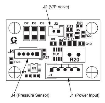
Fig. 36: 249179 Flow Control Board
