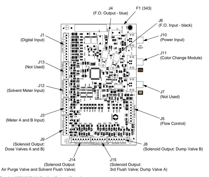
Fig. 21: 255765 Fluid Station Control Board
