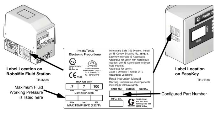
Fig. 2: Identification Label, Automatic RoboMix Fluid Station Systems
