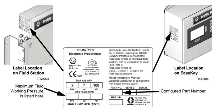
Fig. 1: Identification Label, Automatic Wall Fluid Station Systems
