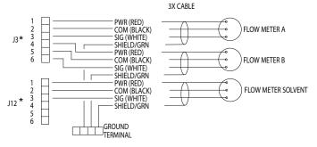
\*Connectors on Fluid Station Control Board
