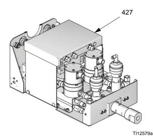
Fig. 27: Remove Control Board Cover
