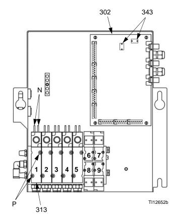
Fig. 22: Replacing Solenoids and Fuse
