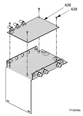
Fig. 28: Remove Control Board
