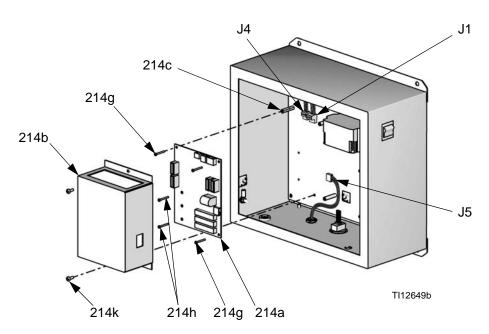
Fig. 17: Replacing Barrier Board
