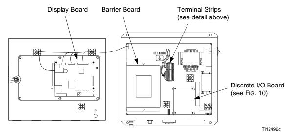
Fig. 9: EasyKey Control Boards and Terminal Strips
