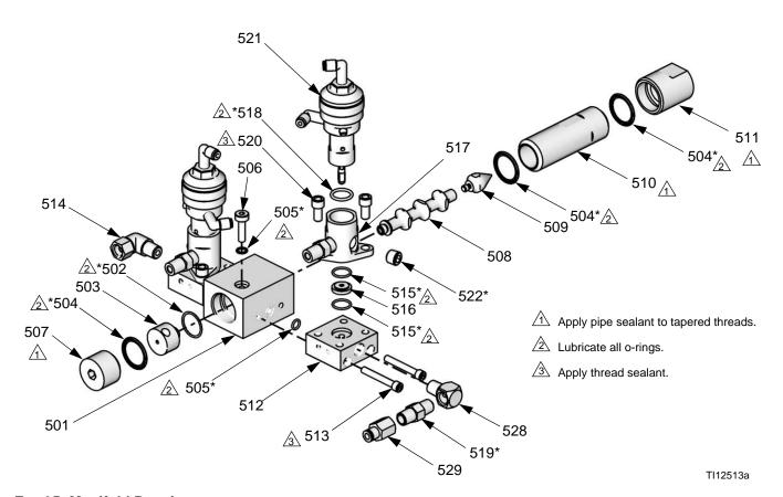
Fig. 35: Manifold Repair
