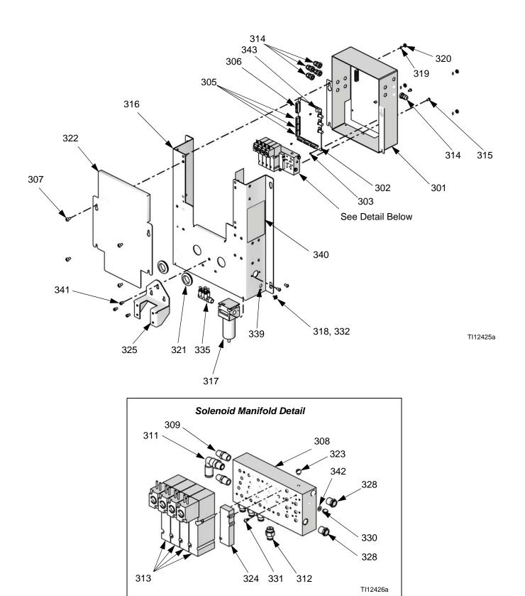
Fig. 20: Wall Mount Fluid Station
