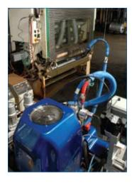
The system's MD2 Dispense Valve and static mixer are mounted to an actuator on the laminating machine that travels back and forth across the nip trough to evenly distribute the mixed material.
