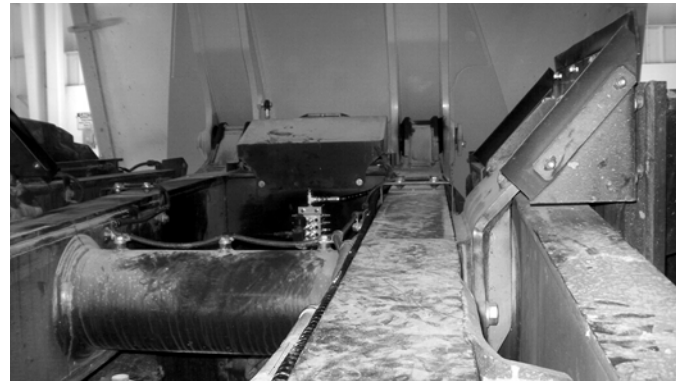
FIG. 110: Master to Rear Secondary Valve supply hose. Routed along left side dump body frame rail to divider valve on HM300-5.
