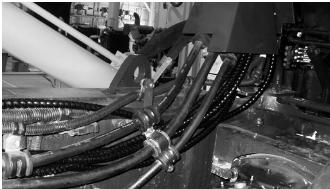
FIG. 107: Hoses left side to left side dump body frame rail on HM300-5.
