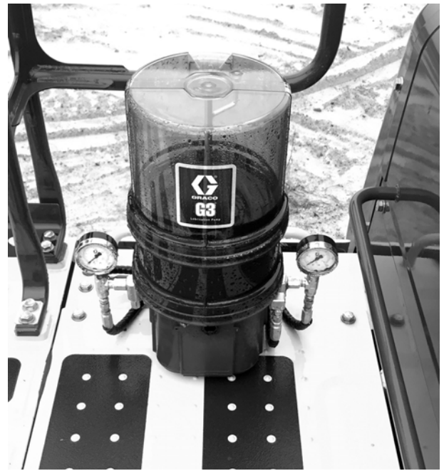
FIG. 32: G3 Pump installed on PC360-11/PC390-11/PC490-11 Models
