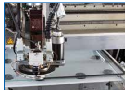
The Graco PGM Metering System provides precision gear metering and ultimate control for smooth, consistent bead and ribbon dispensing. Shown here without hood for better detail.
