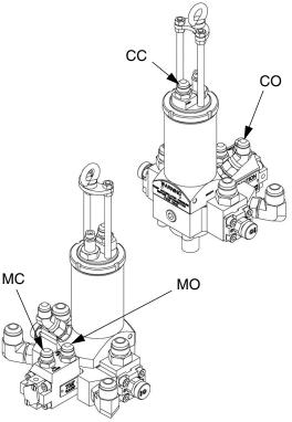
FIG. 8: Hydraulic connections on L-Head
