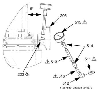
Apply sealant to threads prior to assembly.
