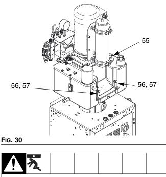
To prevent serious injury from the hydraulic power pack falling, ensure that the hydraulic power pack is secured to the hydraulic lift before removing from the stand.
