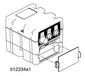
FIG. 36: Remove Access Cover
