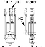
FIG. 9: Hydraulic connections on S-Head
