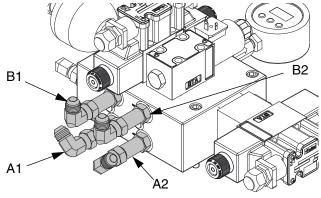
FIG. 6: L-Head Applicator Hydraulic Housing
