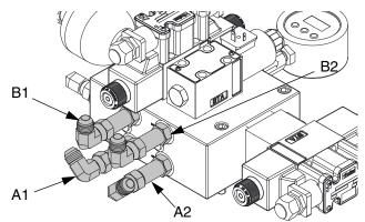
FIG. 26: L-Head Applicator Hydraulic Housing
