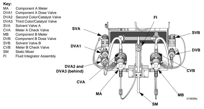
Fig. 2. ProMix 2KE Fluid Controls, Sequential Dosing
