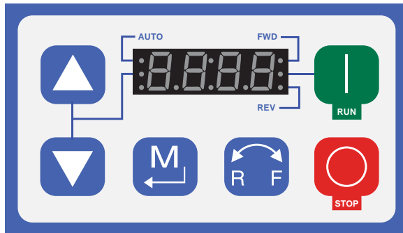
Figure 15 VFD Control Panel
