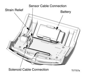
Fig. 1. Battery Location and Module Cable Connections
