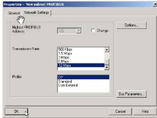
**FIG. 56: Set Transmission Rate**
