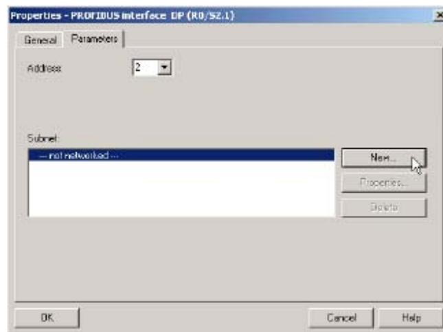
**FIG. 55: Create a New Profibus Network**
