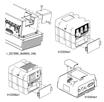
FIG. 13: Remove Access Cover
