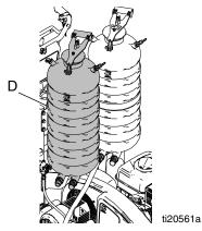
6. Place clamping band (E) around tank and secure with hardware from frame.
