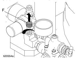
9. Apply thread sealant and install nipple fitting.
