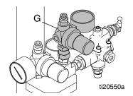
Install 36 in. nylon air line from top of second regulator (G) to swivel fitting on top of second bead tank. Push airline into each fitting as shown.
