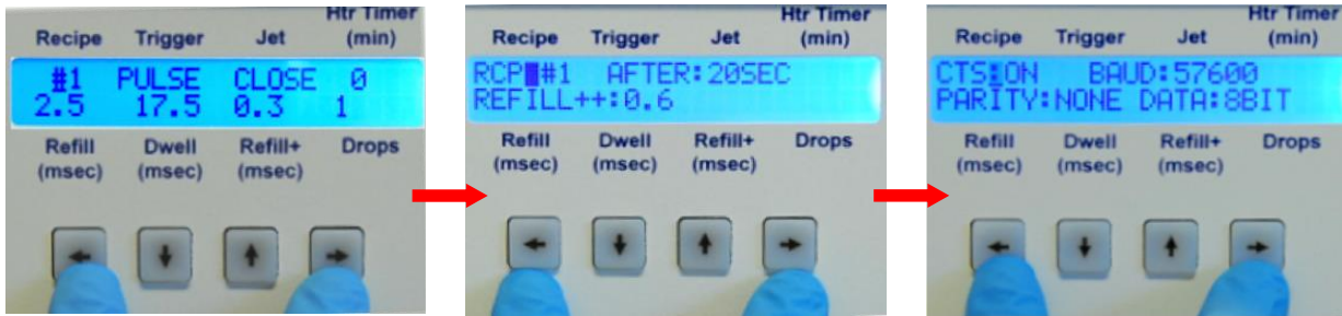
Figure 4-2: Press LEFT+RIGHT Keys Twice for the Default RS-232 Settings
